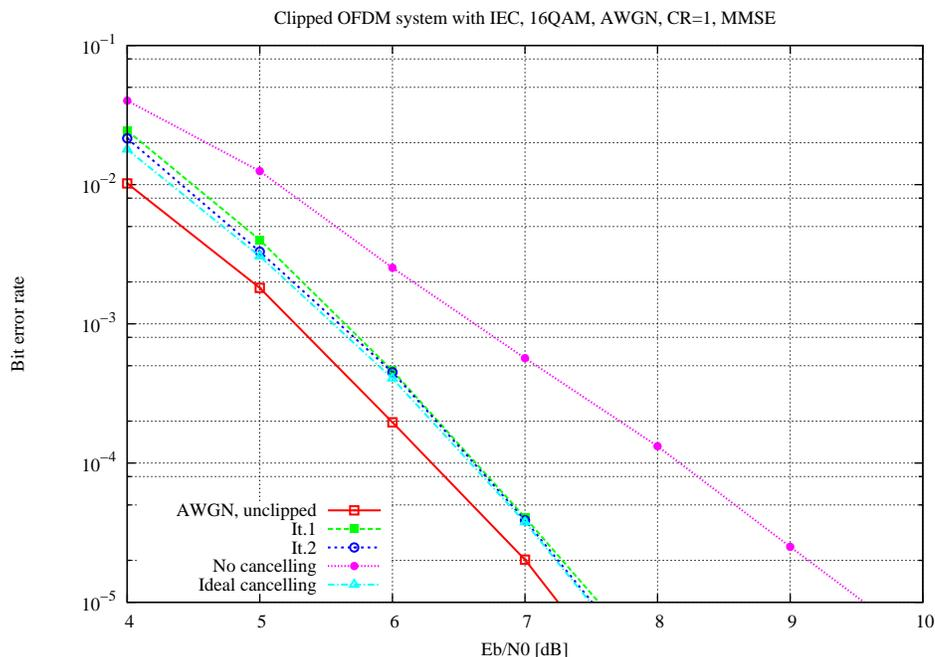
**Figure 4.4.** A simulation similar to that of figure 4.3, with an MMSE equalization instead of zero-forcing.
