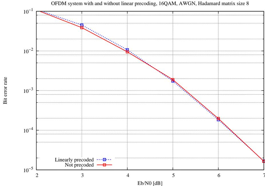
**Figure 3.3.** OFDM system with and without linear precoding using a Hadamard matrix of size 8 over an AWGN channel.
