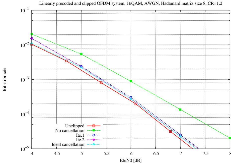
**Figure 4.8.** A linearly precoded, clipped and zero-forcing equalized OFDM system with clipping ratio equal to 1.2.
