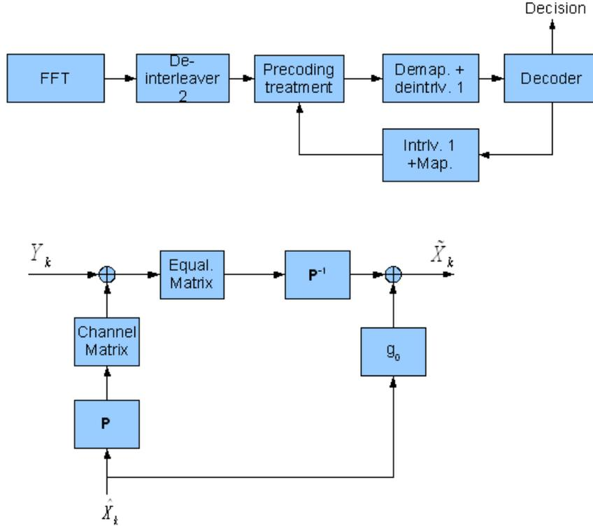
**Figure 4.10.** Block diagram of Le Masson's OFDM receiver with iterative treatment of linear precoding. Above is the general block diagram, and as before, the entrance from the channel into the FFT block is omitted. Below is the definition of the precoding treatment block; inputs and outputs in this figure correspond to those in the general block diagram.
