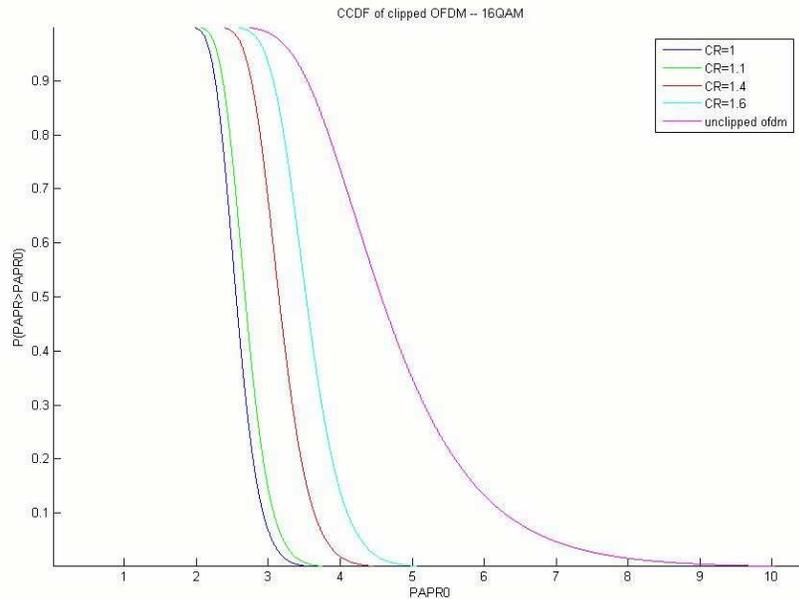
**Figure 2.2.** CCDF of the PAPR of a clipped and filtered OFDM sequence of symbols. In this figure, there is a total of 64 subcarrier frequencies, and the oversampling factor is equal to 16.
