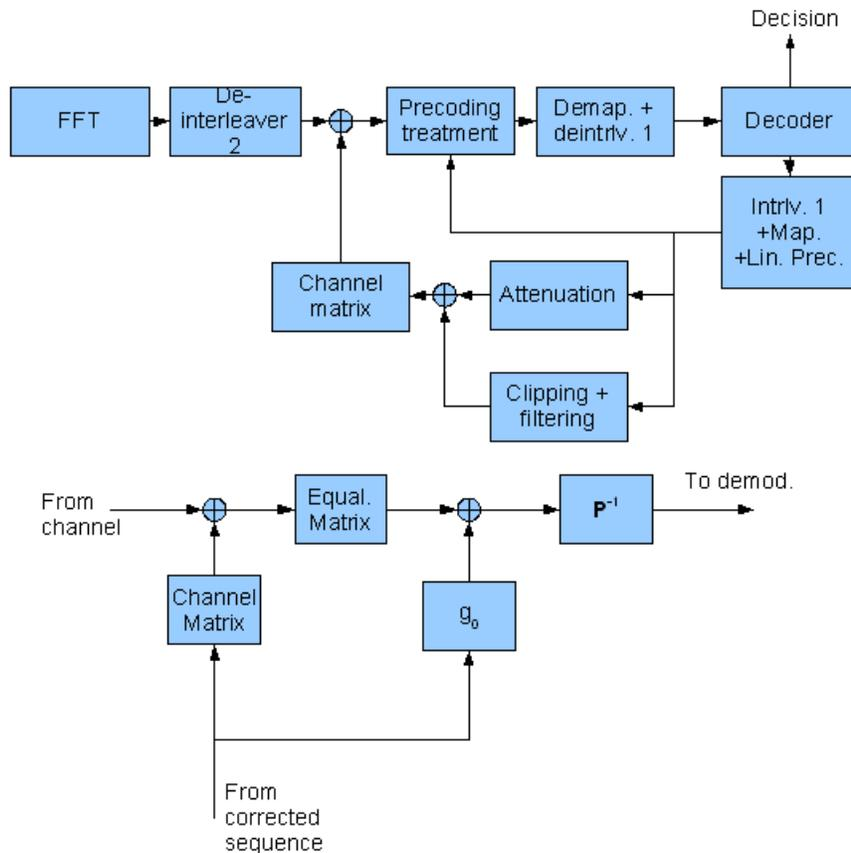
**Figure 1.** Linear precoding treatment as proposed in [3] combined with the IEC technique proposed in [8]. Equalization for the attenuation provoked by clipping is not presented. The above block diagram shows the general structure of the detector, and the block diagram below shows a modified precoding treatment designed to work alongside the IEC branch.
