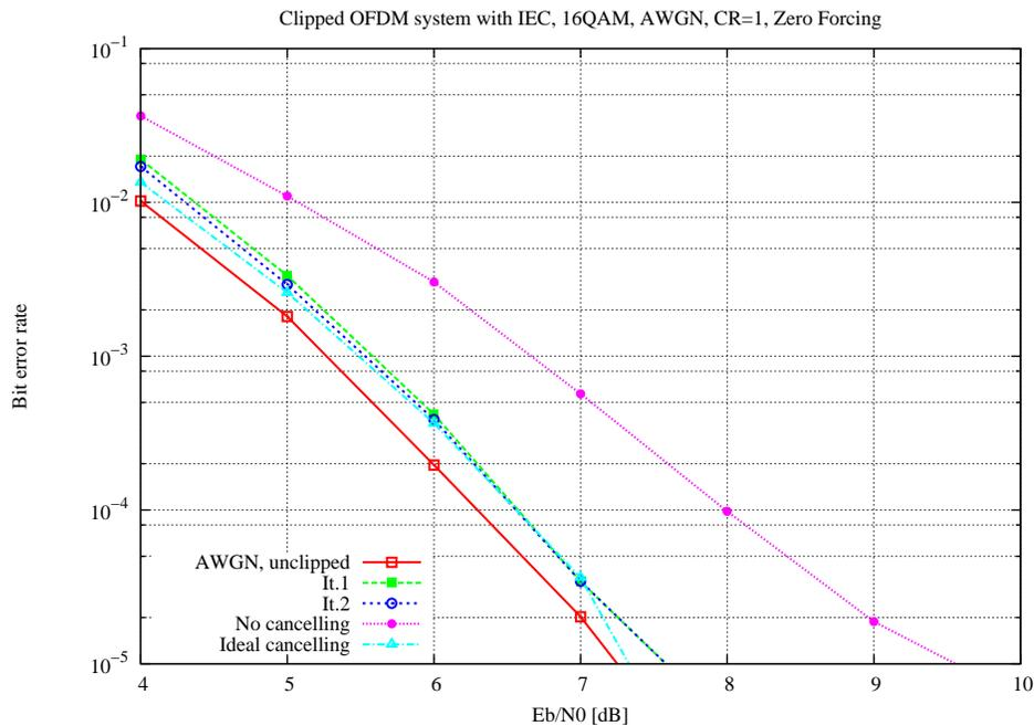
**Figure 4.3.** Reproduction of the simulation shown in figure 4.2, including zero-forcing equalization.
