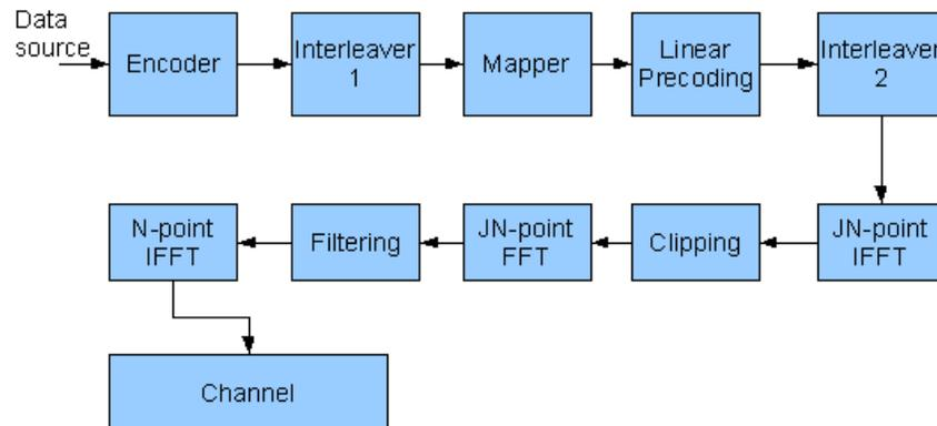
**Figure 3.4.** Block diagram for an OFDM emitter with clipping, filtering and linear precoding. The receiver is the same as the one used for a linearly precoded OFDM system.
