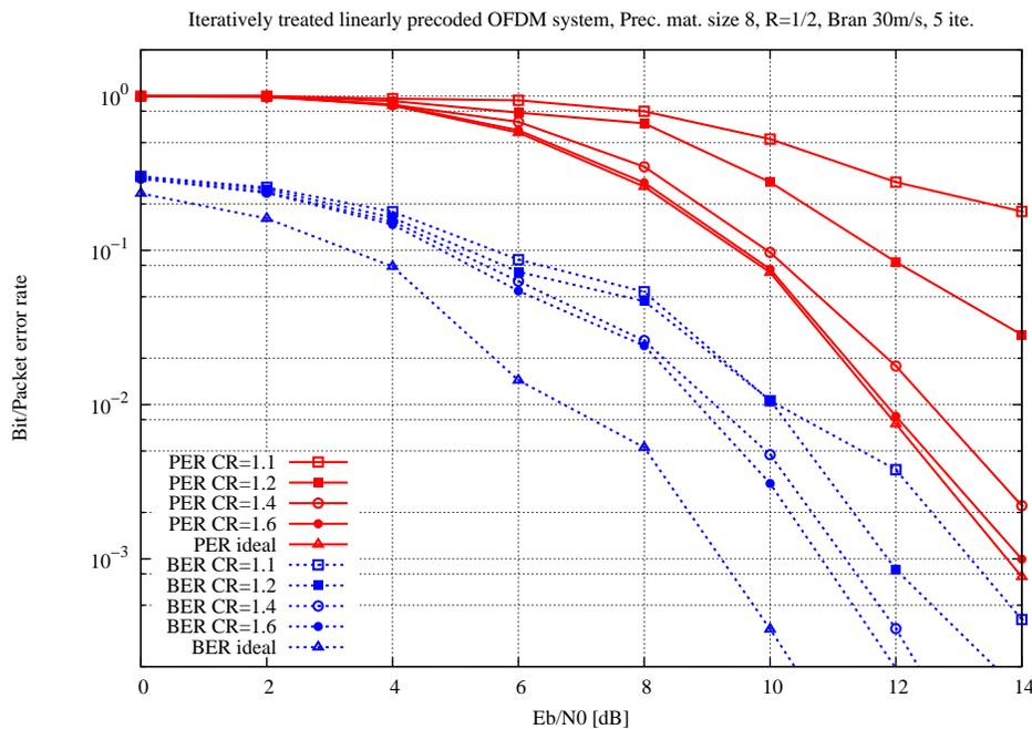
**Figure 4.11.** Clipped and precoded OFDM transmitter tested with J. Le Masson’s iterative linear precoding treatment receiver over a multipath fading channel. Packet error rates worsen as the CR drops below 1.6.
