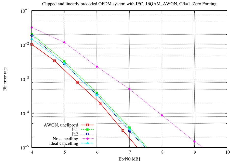
**Figure 4.6.** Linearly precoded and clipped OFDM system with zero-forcing equalization.
