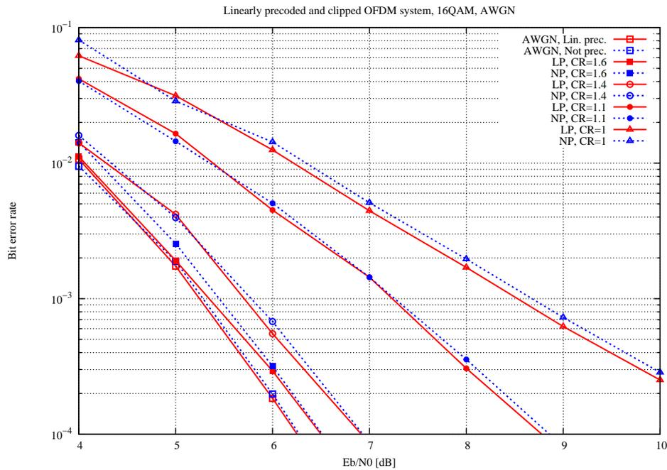
**Figure 3.5.** Performance of a precoded and clipped OFDM system for a variety of clipping ratios. As mentioned before, the linearly precoded and non-precoded unclipped system's performance curves are identical. They are shown from this point on for the sake of completeness.
