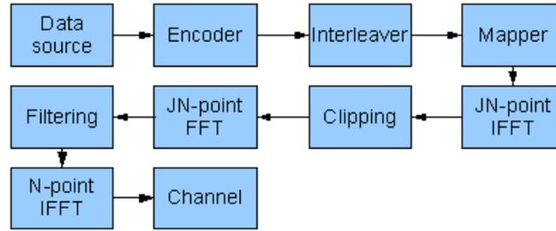
**Figure 2.1.** Block diagram for an OFDM transmitter that includes oversampling, clipping and filtering as shown on the second row.
