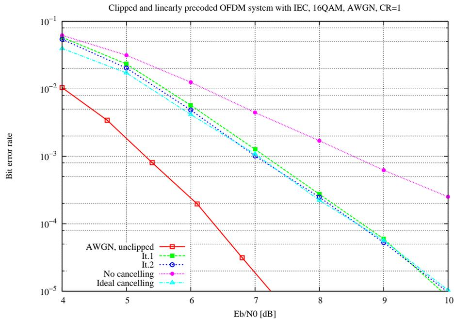
**Figure 4.5.** Clipped OFDM system with parameters equal to those of fig. 4.2 and including linear precoding.
