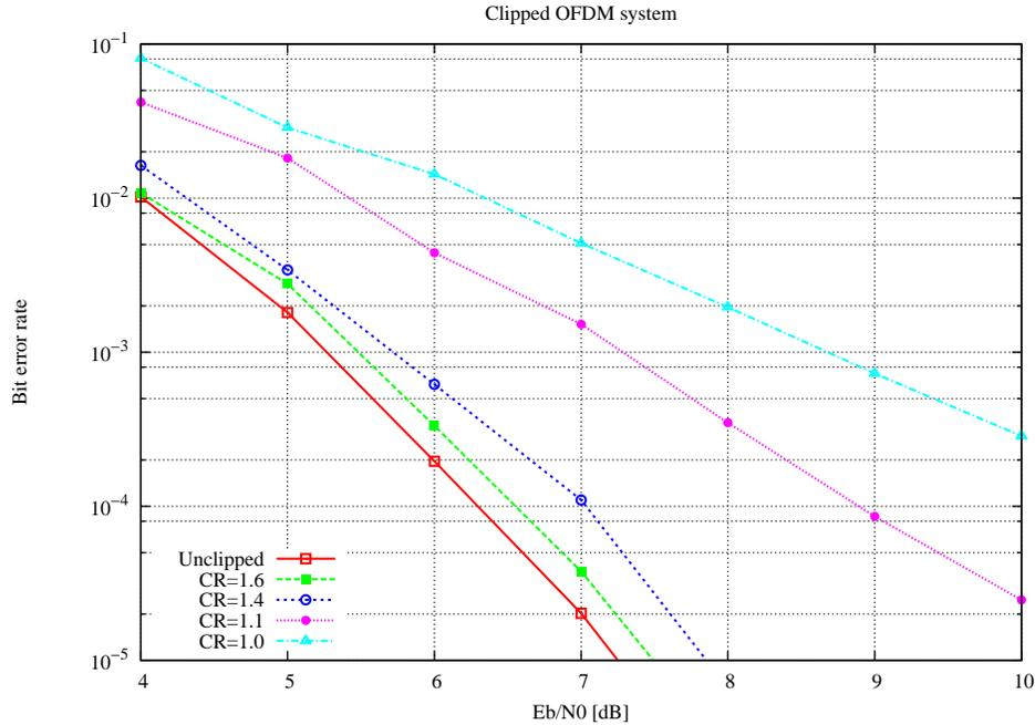
**Figure 2.3.** System performance for 64 subcarrier frequencies, oversampling factor of 16 and the shown clipping ratios over an AWGN channel. Performance worsens as the clipping ratio is reduced.
