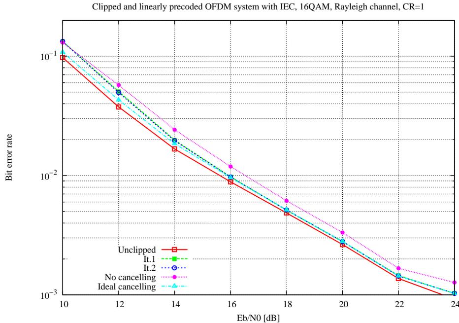
**Figure 4.9.** Clipped OFDM system with linear precoding, IEC and zero forcing equalization over a 16-path white Rayleigh channel. The clipping ratio is set to 1.
