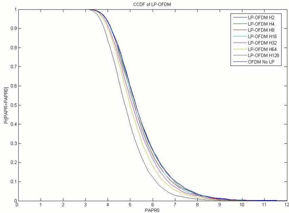
**Figure 3.2.** CCDF of linearly precoded OFDM PAPR using Hadamard matrices. As seen above, as the precoding matrix is chosen larger, the CCDF curve shifts to the left, showing a reduction of PAPR.
