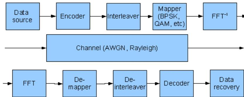
**Figure 1.1.** A simplified OFDM transmission chain. Right before and after the channel are the DFTs who provide the core for this type of modulation. Some details, like transmission filters and guard interval insertion, are implicit while others are made explicit for the first time.
