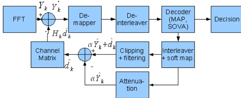
**Figure 4.1.** IEC-implementing clipped-OFDM receiver. The entrance of information from the channel into the FFT is not shown in the figure.
