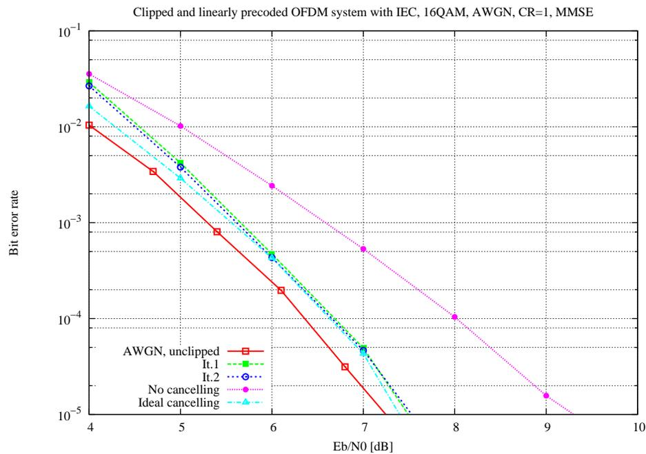
**Figure 4.7.** Linearly precoded and clipped OFDM system with MMSE equalization.
