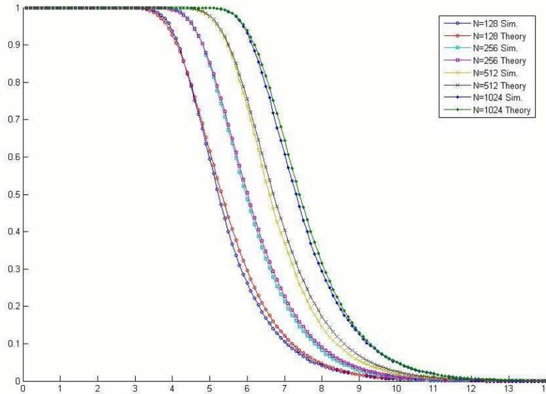
**Figure 1.2.** CCDF of PAPR for a given number of subcarrier frequencies. On the  $x$  axis, the possible values of PAPR are shown, while the  $y$  axis represents the probability of finding a PAPR larger than the value considered in  $x$ . Both axes are dimensionless. (Taken from [4])
