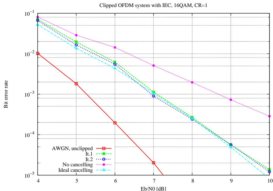
**Figure 4.2.** OFDM system clipped with CR=1. There is a significant improvement in performance, but the non-clipped system's curve is far from being reached.
