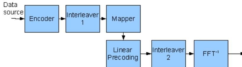
**Figure 3.1.** A simplified precoded OFDM transmitter. A new interleaver provides added protection against burst errors and minimizes any existent correlation between subsequent symbols.
