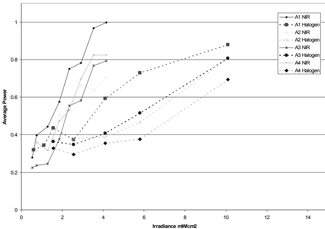
Fig. 10. Average power of the signals obtained from the velocity sensor (silicon photodiode) in **Arteries**. It is possible to register the same average power with NIR using one third as much irradiance than halogen lamp irradiance.
