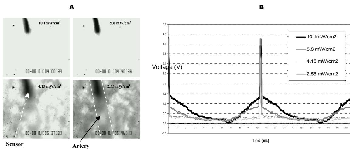
Fig. 6. Comparison between correlation peak and the corresponding image captured with the camera using *halogen lamp*. A) Image obtained for each irradiance. B) Correlation signal for each irradiance .
