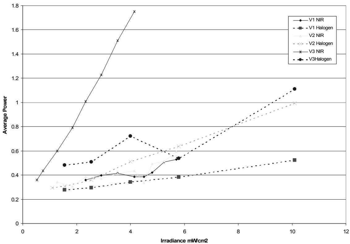
Fig. 11. Average power of the signals obtained from the velocity sensor (silicon photodiode) in *veins*. The NIR presents a higher average power in comparison to the halogen lamp.
