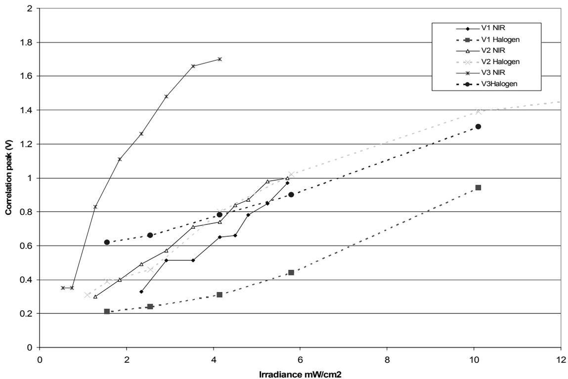
Fig. 9. Magnitude of the cross correlation response with different irradiance for NIR and Halogen lamp in veins .
