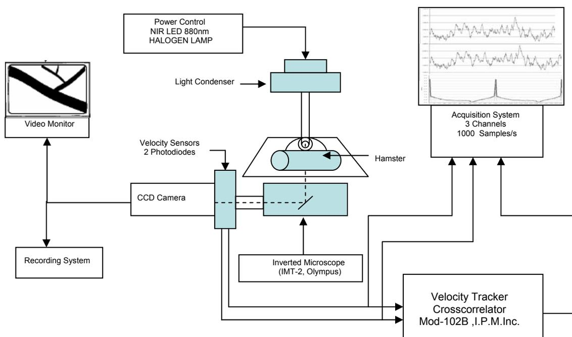
Fig. 1. Schematic diagram of the experimental setup. A personal computer with Analog to digital converter was used to acquire the three signals for the analysis of signal average power and delay correlation.
