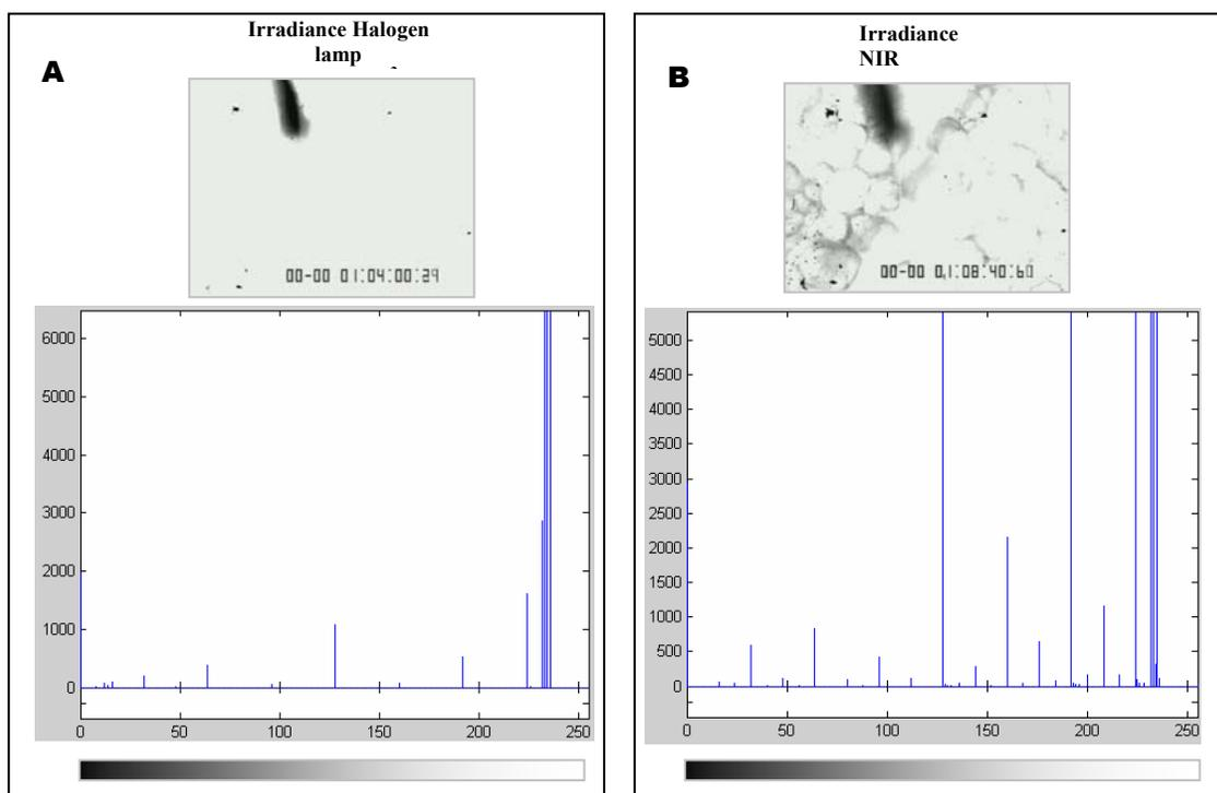
Fig. 12. Histogram of the images at the 1.35 V level of the peak in cross correlation response . A) Image and histogram for the halogen lamp irradiance . B) Image and histogram for the NIR . The NIR image shows the fat cells and the artery in the velocity measurement without saturate the image , in contrast with halogen lamp that need of high energy to find cross correlation with the photodiode sensors.
