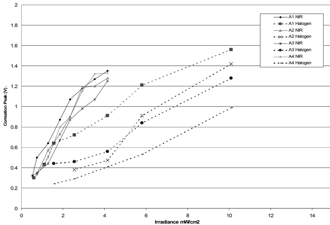
Fig. 8. Magnitude of the cross correlation response with different irradiance for NIR and Halogen lamp in arteries.
